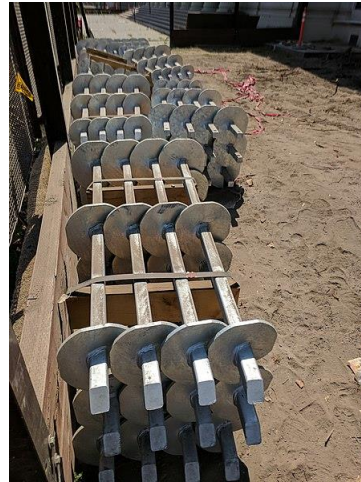
Fig.25 : Example of screw pile (Wikimedia Commons, licensed under CC BY-ND 2.0)
