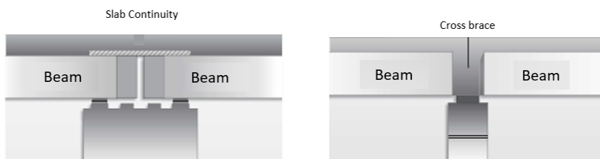
Fig.12 : Longitudinal section (precast reinforced concrete beams)
